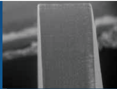
B- Edge profile. Radius of curvature < 10 \mu\text{m} .
